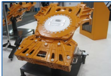
JVS - Articulation system IK59B for the low-floor buses allowing for bend angles of \pm 54^\circ , pitch angles of \pm 10^\circ and torsion angles of \pm 3^\circ .
