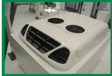
WEBASTO - The new series of water heaters Thermo Top Pro 120 and Thermo Top Pro 150 of 12 and 15 kW and Cool Top 110 RT-CS climate group for mini and midibuses, with 11 kW of cooling capacity and 12 kW of heating capacity.
