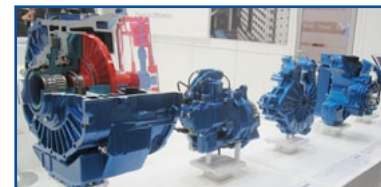
VOITH - From Diwa.6 automatic transmission with Stop-Start to a secondary water retarder and air compressor equipped with 'TwinSave' technology.
