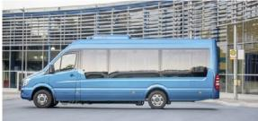
The lowered frame between the axles is facilitating the use in regular-service operations and the lowered section covers a surface of approximately 3.5 m<sup>2</sup>. The total weight of 5,650 kg provides the necessary weight reserves for carrying up to 30 passengers.
