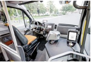
The panoramic windscreen with integrated destination display stretches right up into the roof, while the vehicle sides are extensively glazed and the belt line low. The overall effect is light and aesthetically pleasant.
