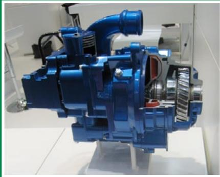
The DIWA automatic transmission was specifically developed for buses. Compared with its predecessor model, the DIWA.6 can save almost another 5% fuel. Apart from utilizing the topography-dependent program SensoTop, this is made possible by the need-based reduction of the operating pressure and an intelligent start-up management.
