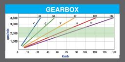
The tested vehicle has the electro hydraulic automated Mercedes NAG W5A 380 with five speeds. Transmission Ratio 4.182
