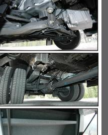
axles, which eliminates any hint of pitching. The rest of the work is performed by the sturdy mechanical suspensions (independent wheel on the front), which can optionally be replaced by pneumatic rear axle suspensions to further enhance passengers' comfort.
